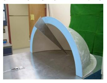
Figure 3: Reflector of a Prolate-Spheroidal IRA
