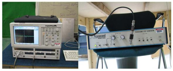
Figure 4: Sampling-Oscilloscope and pulse Generator
