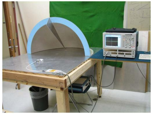
Figure 2: Experimental Setup for a Prolate-Spheroidal IRA
