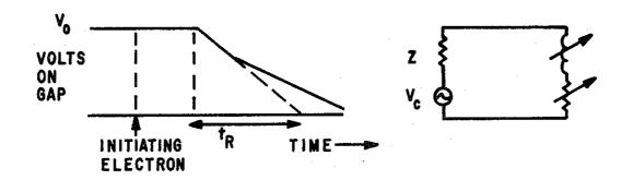
In the experiments with gas sparks transmission lines (or cables) of 100, 10 and 1 ohms were used and spark channel fields of 3 x  $10^4$  down to 5 x  $10^3$  volts/cm were used in air. Other pressures than atmospheric were employed and also gases of other densities. From these experiments (supported by the calculations) the following relation for the resistive phase was obtained:
