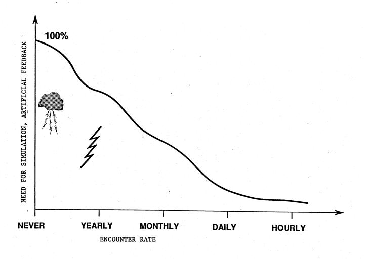
FIGURE 1. Illustrating the increasing need for testing in simulated environments with decreasing frequency of encountering the threat
