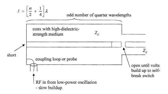
Consider fields in coax as superposition of left and right going waves. When the switch closes the wave propagates out to right.
