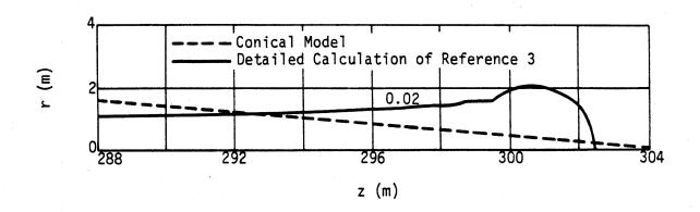
Figure 2. Comparison of the predicted tip geometry for both the conical model of this note and the more detailed calculations of Reference 3.
