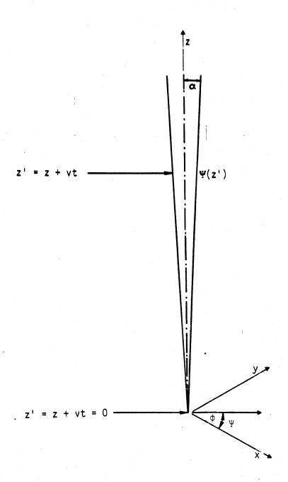
Figure 1. Triangular tip for leader moving at velocity v.
