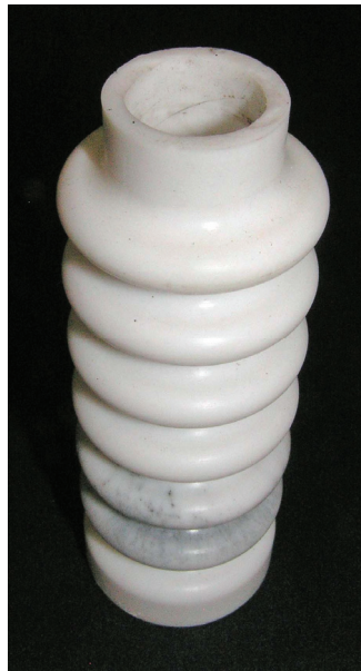
Figure 25. Gas Discharge Tube for high power experiments.
