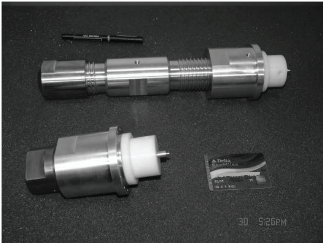
Figure 13. Switched oscillators (200 MHz top) and 500 MHz (Bottom)
