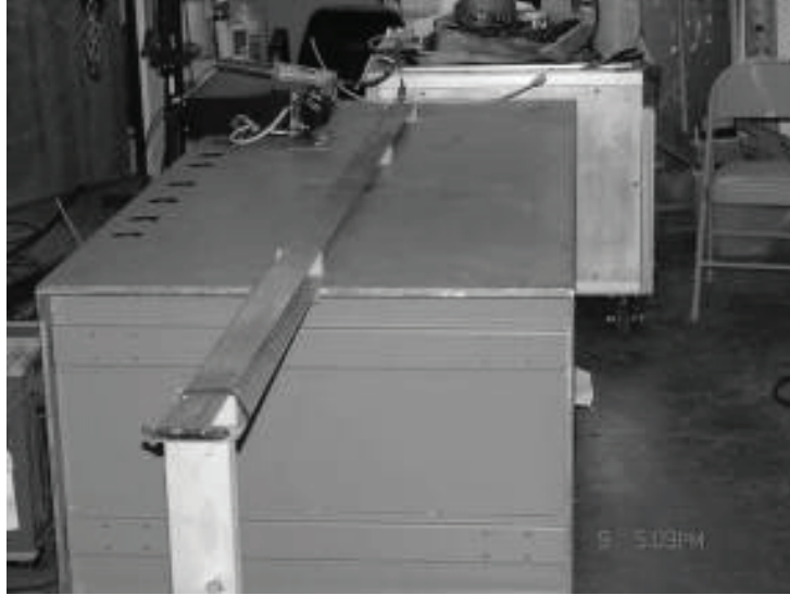
Figure 14. Switched oscillators tested into a 100 \Omega dummy load transmission line
