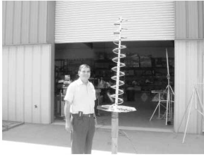
Figure 23. Illustration of the helical antenna and the associated octagonal ground plane
