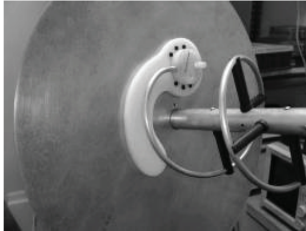
Figure 34. Switched oscillator/antenna interface and the measured S_{11}
