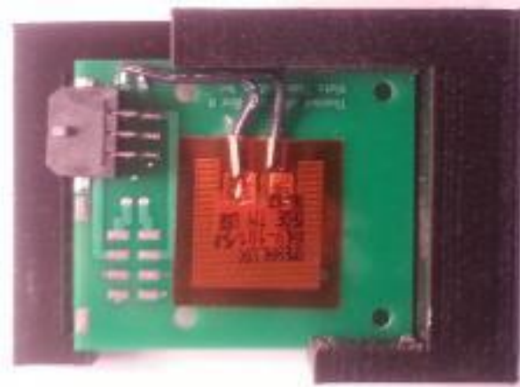
Temperature controlling Peltier NanoCards with built-in thermistors.
