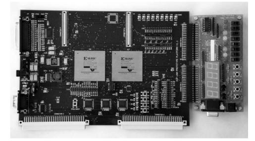
**Figure 1** The completed XUP–UNM platform with matted Digilent I/O board is shown here. By co-ordinating the design effort with the Digilent Corporation, interfacing with their series of peripheral input and output boards was accomplished. Their boards possess the capabilities including ADC, DAC, wire wrapping, and LCD.
